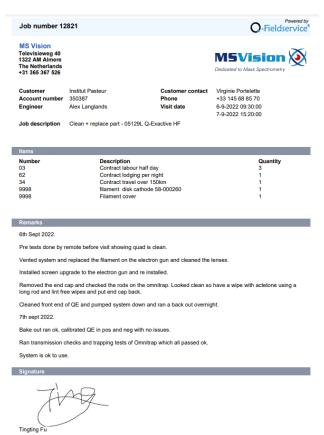
**Figure 1.** Field service activities provided by MSVision in collaboration with Fasmatech to reinstate the performance of the omnitrap platform installed at Institut Pasteur.
