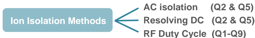
Figure 3. The different ion isolation methods available in Q2 and Q5 include the application of AC waveforms, the application of a resolving DC similarly to the operation of a quadrupole mass filter as well as controlling the duty cycle of the rectangular RF waveforms.
