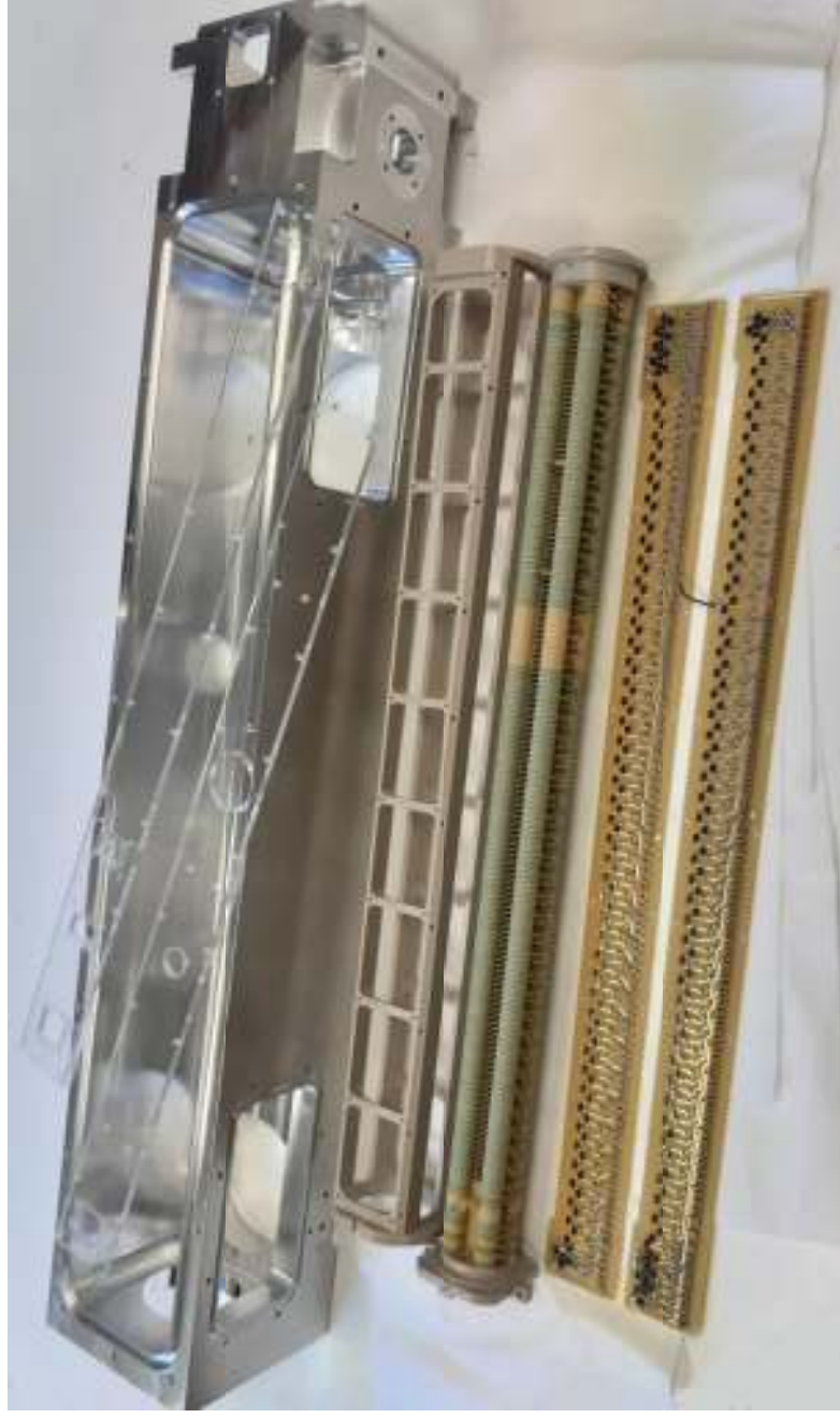
IMS outer & inner housing, drift pcb-electrode assembly, vacuum pcb's and electronics circuitries
