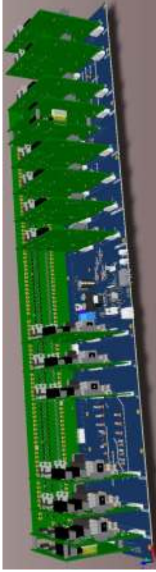
IMS Switch Board & Floating Switch Cards
