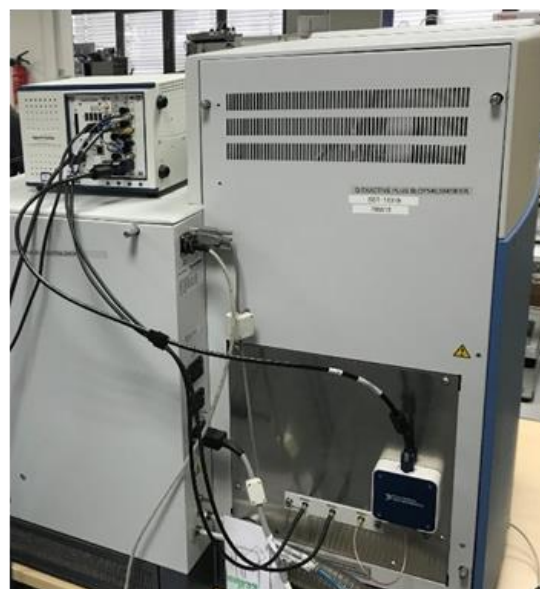
Figure 7.1. Prototype FTMS Booster TD: (top panel) shows new-generation type architecture of this high-performance data acquisition system; (bottom panel) shows a general picture of a device and its installation on a Q Exactive UHMR Orbitrap FTMS performed at a TopSpec partner site (TFS, Bremen, Germany). The interface of connecting FTMS Booster TD to an Orbitrap FTMS is visible at the right bottom corner – it includes 2 signal cables originating at the pre-amplifier of an Orbitrap and a trigger cable that operates the FTMS Booster TD as a guest system, whereas Orbitrap acts as a host.
