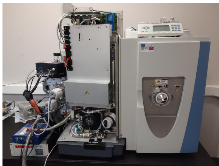
Figure 6.2. Q Exactive HF interfaced with the Omnitrap.
